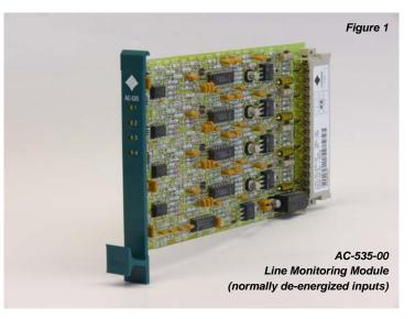
The input connections are guarded against interruption and short-circuiting, each circuit having a front indication. The logic input will be disabled in case of a line short. This function can be disabled per channel. In this case the module acts as an AC-534-B.
