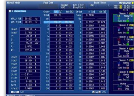
Harmonic components of input signal
