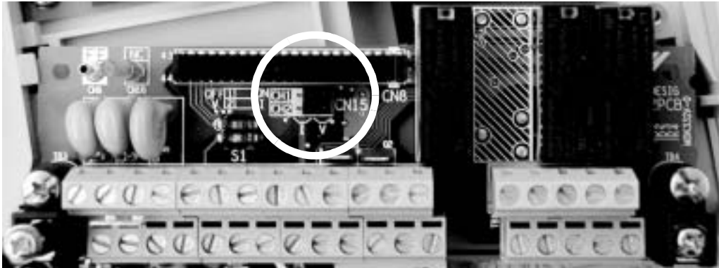
Fig 2.12 Shunt Connector CN15 Location
