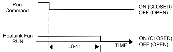
Fig 5.38 Heatsink Cooling Fan Operation Timing Diagram
