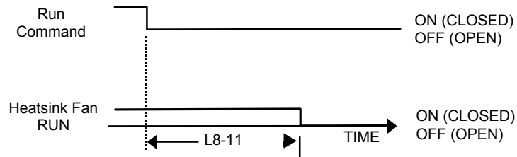
Fig 5.38 Heatsink Cooling Fan Operation Timing Diagram
