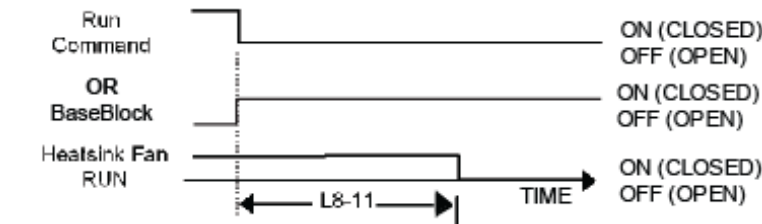
Figure 5.49 Heatsink Cooling Fan Operation Timing Diagram
