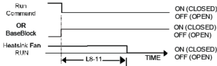
Figure 5.49 Heatsink Cooling Fan Operation Timing Diagram
