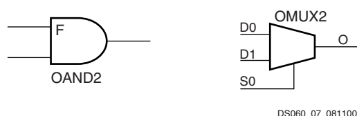
Figure 7: AND and MUX Symbols in Spartan-XL IOB
