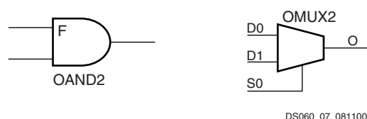
Figure 7: AND and MUX Symbols in Spartan-XL IOB
