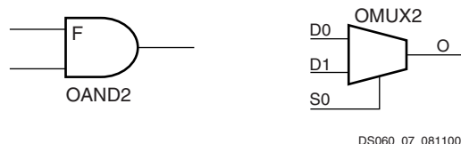
Figure 7: AND and MUX Symbols in Spartan-XL IOB
