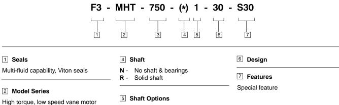
**3** Theoretical Torque in Lb. Ft. per 100 PSI Differential Pressure
