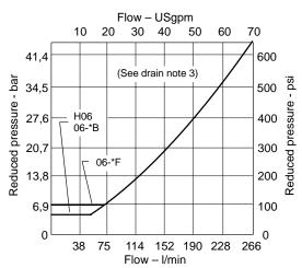
Note: These charts are based on the inlet pressure being at least 10,3 bar (150 psi) higher than the outlet reduced pressure.
