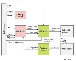
The safety approach of the PVED-CX4 is based on self- and neighbor-monitoring combined with the ability to shut down all neighbor modules. Spool movement, internal electronics, and software processes are redundantly monitored.
