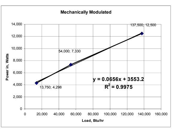
The equations characterizing the compressor power input vs. load is reflected on the figures along with the degree of fit  $R^2$ . The equations were employed in the simulations.
