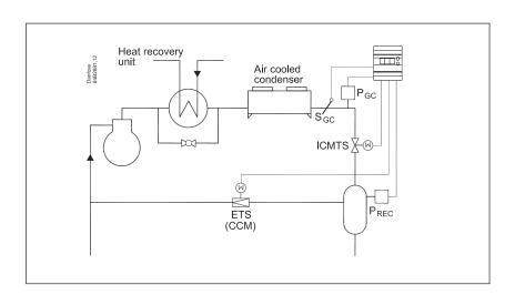
Heat recovery system (or heat pump system)
