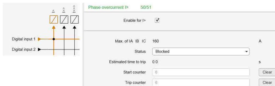
Figure 330 - A view from the setting tool showing a DI input blocking connection (left picture) and the result for the 50/51 stage when the DI is active and the stage exceeds its current start value
