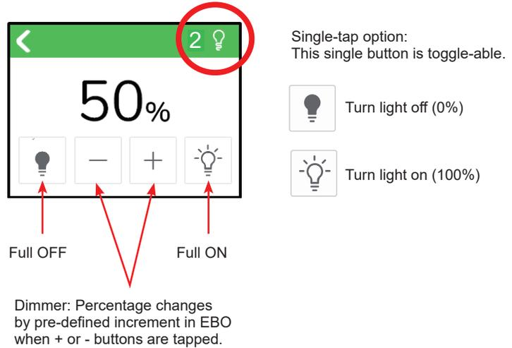
The Full OFF and Full ON buttons allow the light to be turned fully off or on in the group.
