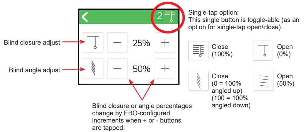
The upper row of buttons controls the closure of the blinds. The lower row of buttons controls the blind angle adjustment.
