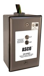
The **ASCO Model 331** surge suppressor is designed for use with AC distribution panel circuits or 120V power supplies feeding sensitive electronic equipment. Electrically, the unit incorporates MOV fusing technology. The Model 331 SPD is designed to be installed in parallel on standard split phase 120/240 VAC (3W+G) or single phase 120 VAC (2W+G) circuits.
