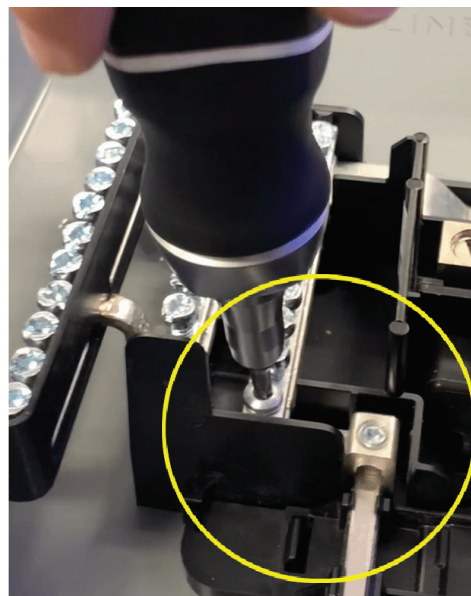
Figure 7 – Inspect for Movement on the Left PoN Connector
