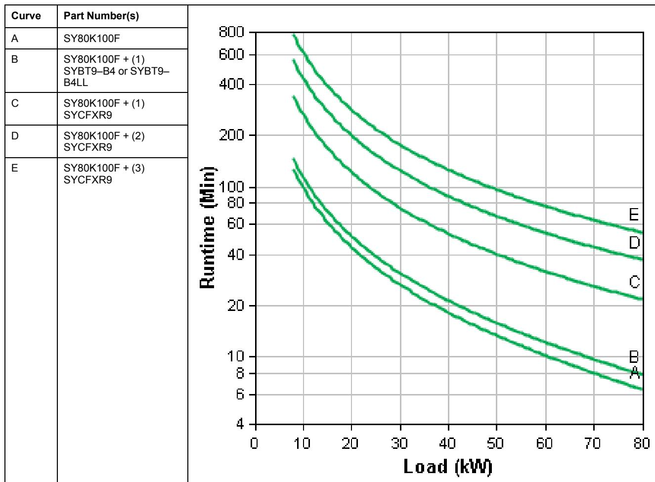
**Symmetra PX 90 kW Scalable to 100 kW Battery Run-Times (Minutes)**
