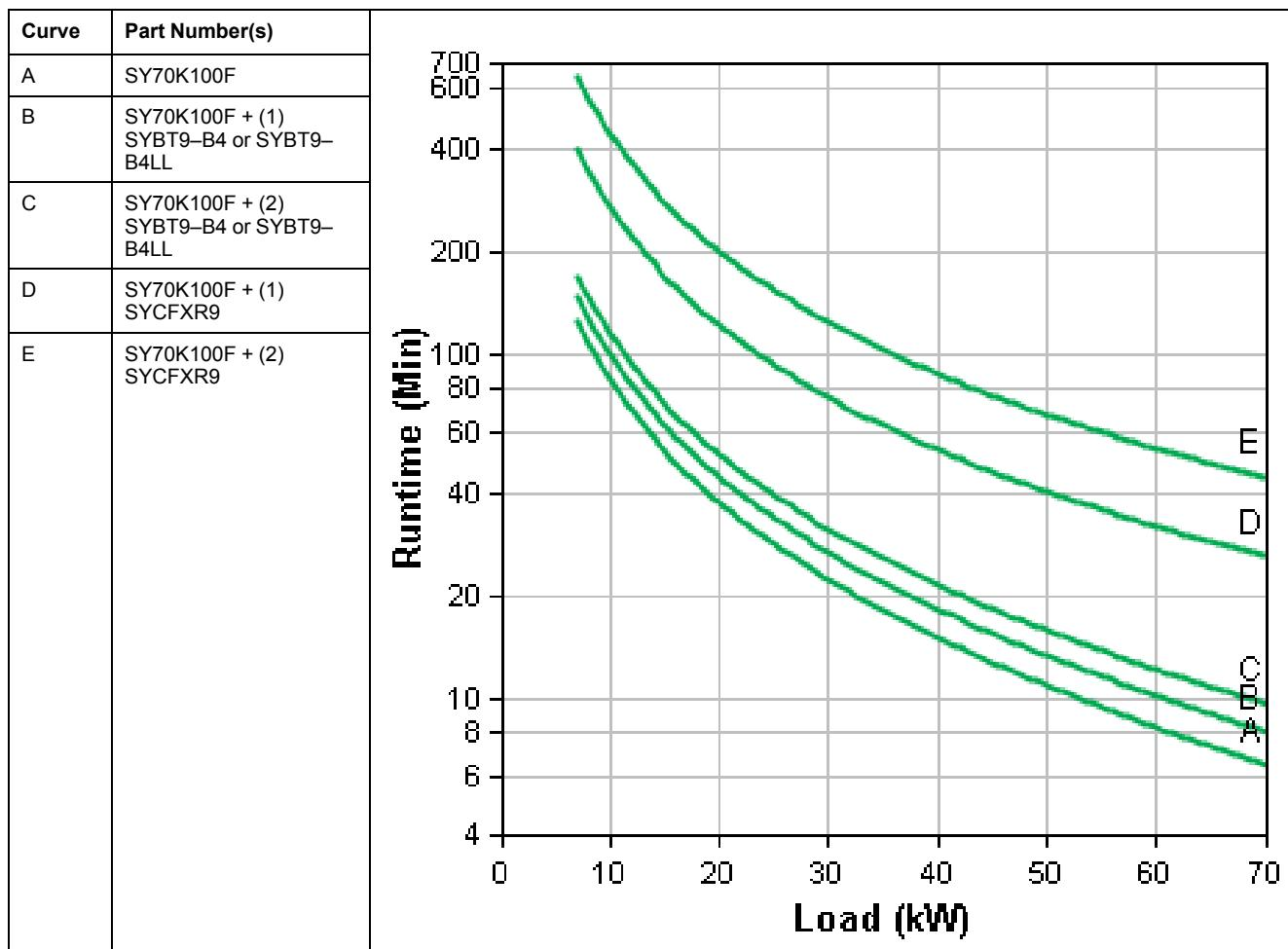
**Symmetra PX 80 kW Scalable to 100 kW Battery Run-Times (Minutes)**
