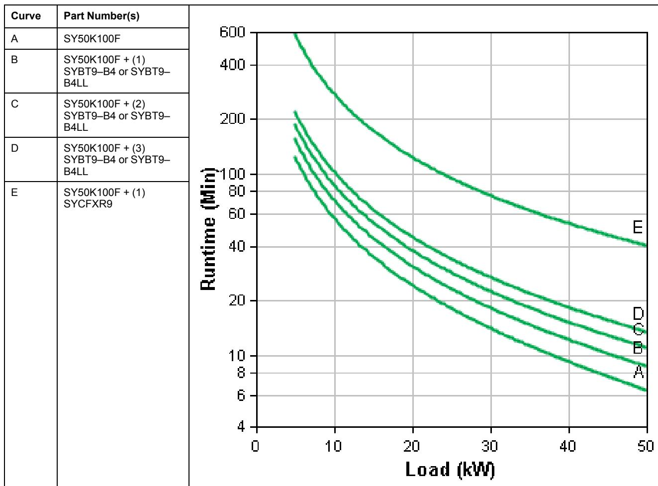
**Symmetra PX 60 kW Scalable to 100 kW Battery Run-Times (Minutes)**
