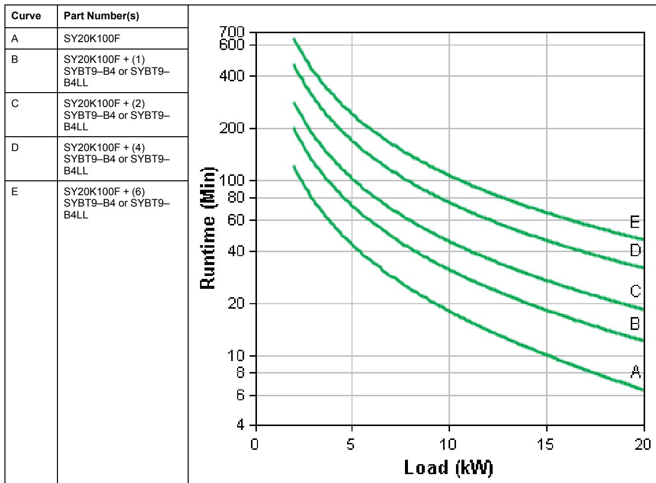
**Symmetra PX 30 kW Scalable to 100 kW Battery Run-Times (Minutes)**
