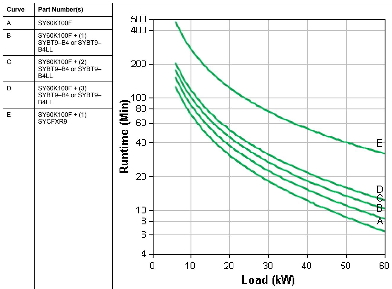
**Symmetra PX 70 kW Scalable to 100 kW Battery Run-Times (Minutes)**
