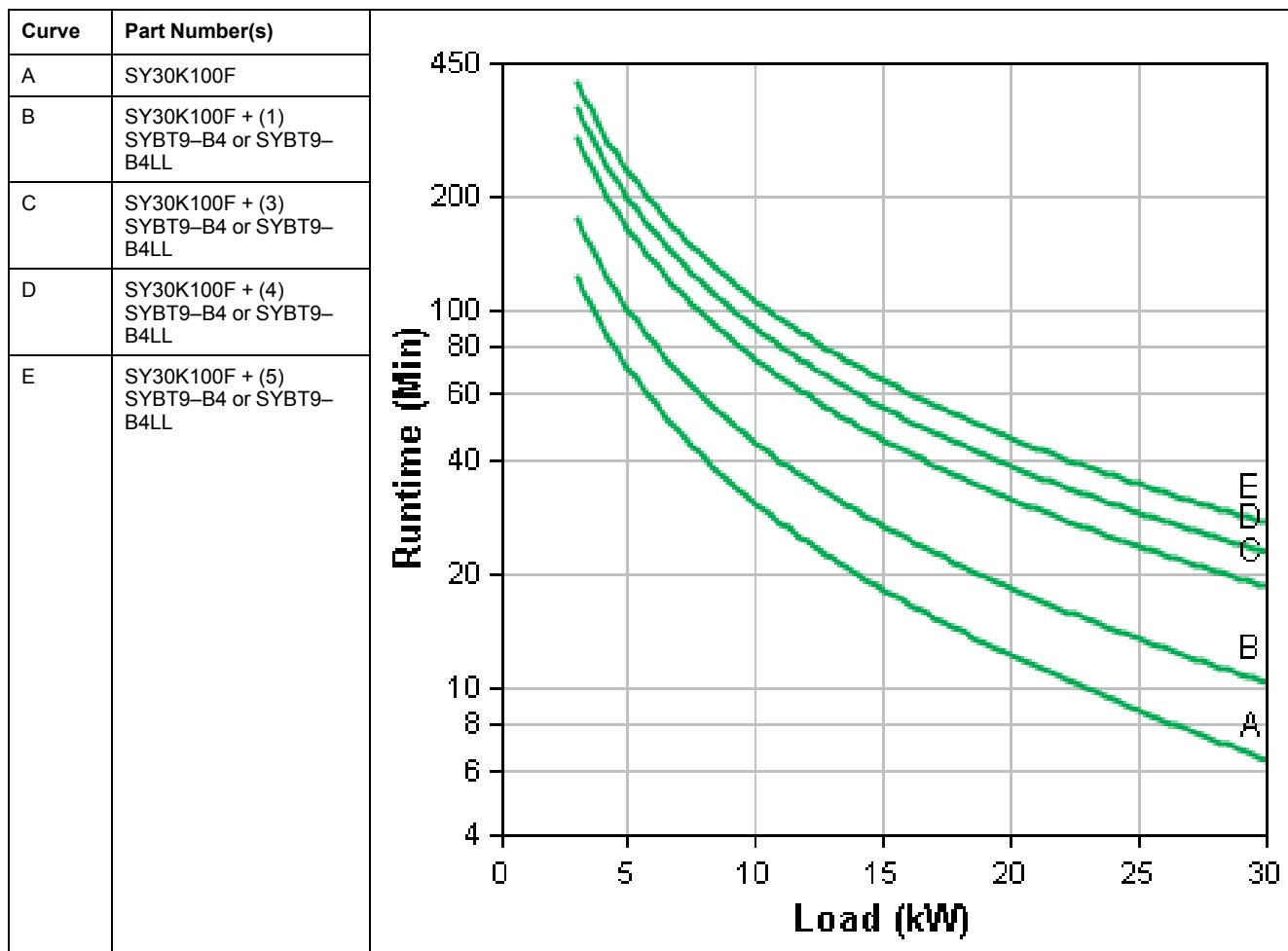
**Symmetra PX 40 kW Scalable to 100 kW Battery Run-Times (Minutes)**
