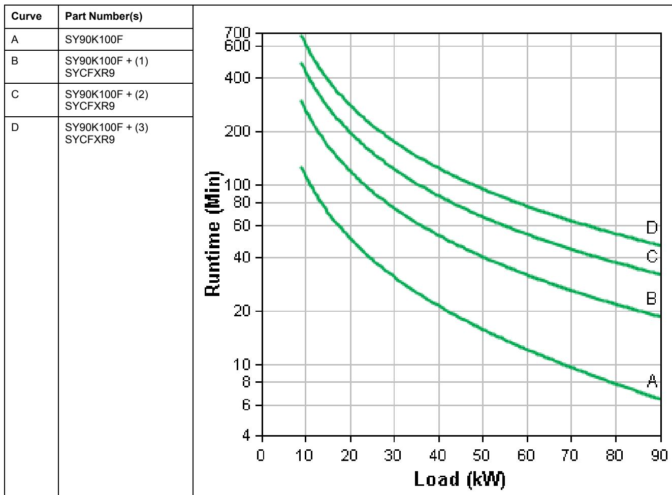
**Symmetra PX 100 kW Battery Run-Times (Minutes)**
