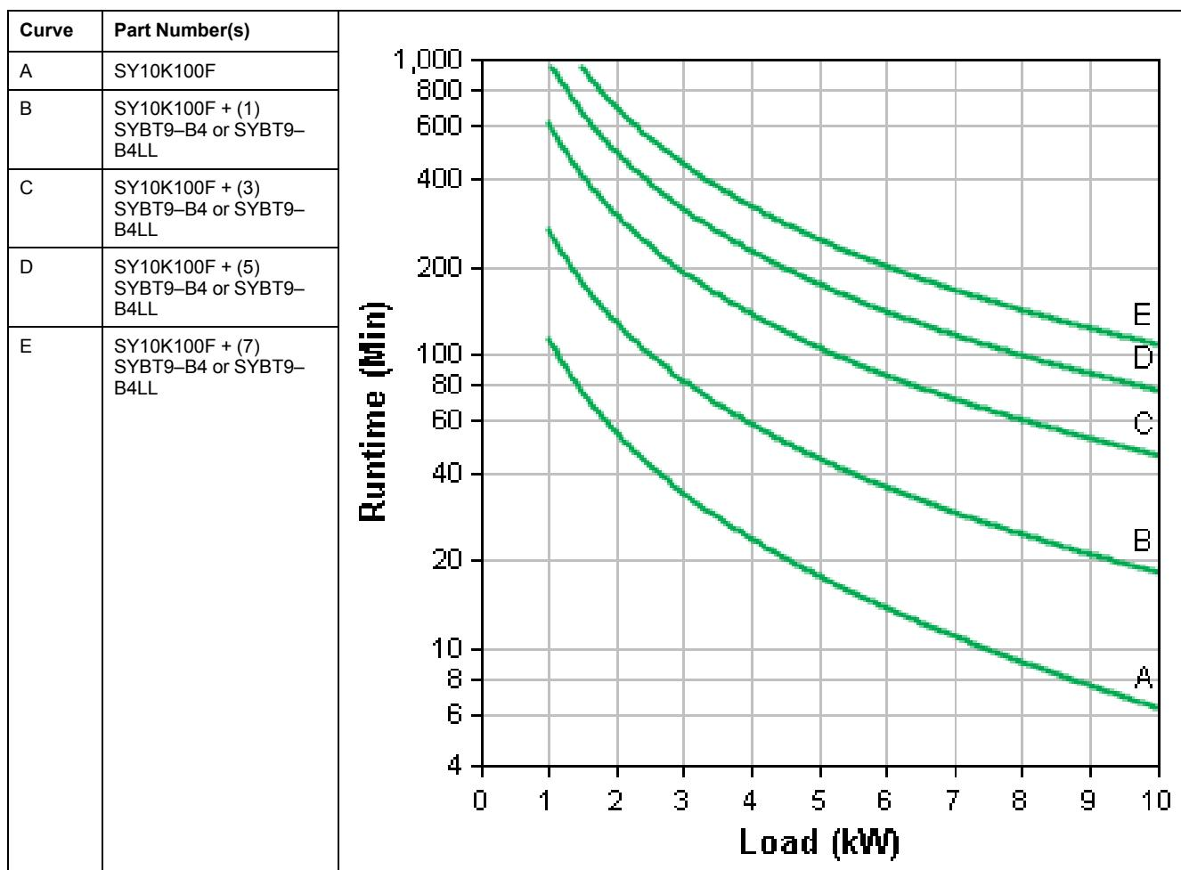
**Symmetra PX 20 kW Scalable to 100 kW Battery Run-Times (Minutes)**
