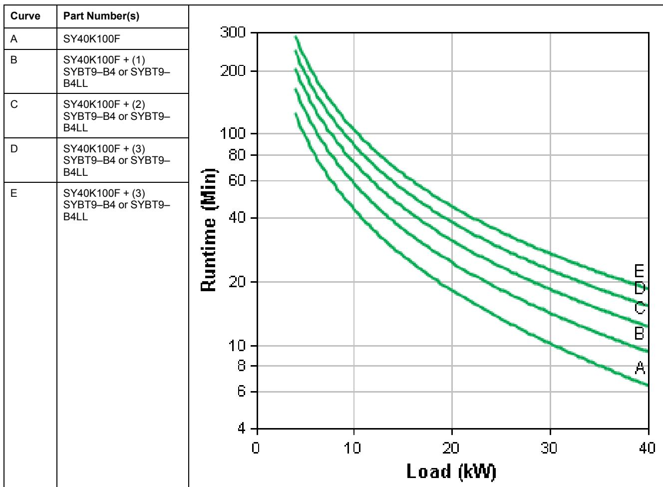
**Symmetra PX 50 kW Scalable to 100 kW Battery Run-Times (Minutes)**
