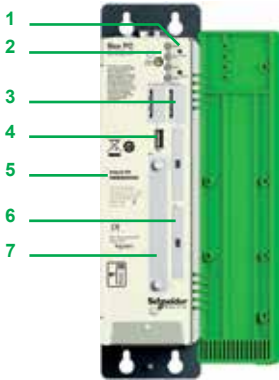
Front panel of Magelis BOX PC, door open 1 PCI slot
