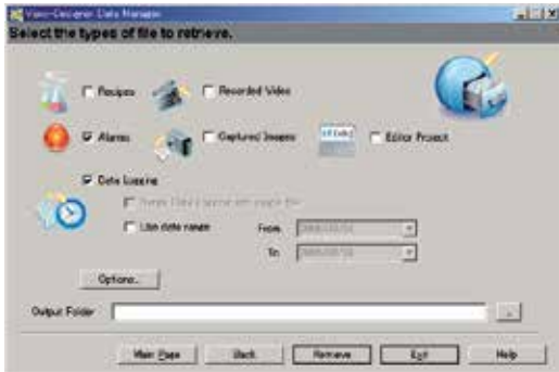
Data Manager: Transfer recipes, videos, images, etc. via Ethernet or USB, by simply clicking the mouse
