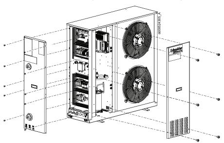
3. Install the VFD fan heater to the VFD cover with two M4 screws.
