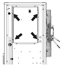
5. Fix the assembled VFD fan heater kit to the outdoor unit with two M4 screws.
