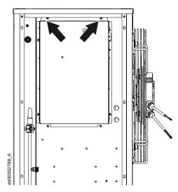
6. Fix power cable to the hole with a wire tie (position A).
