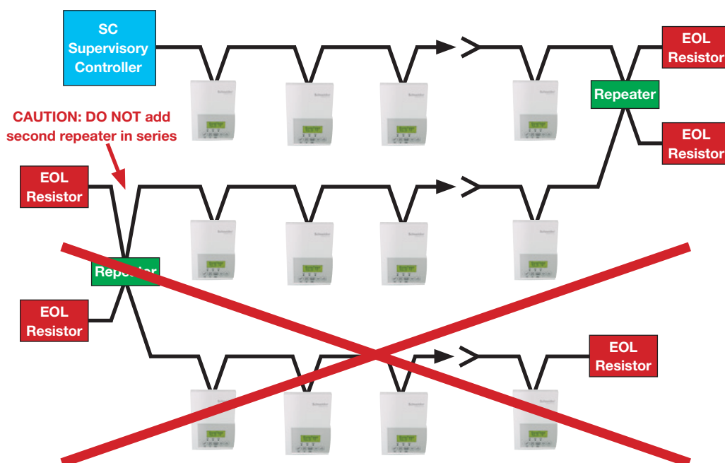
Figure-6 Incorrect Repeater Use in an EIA-485 Network
