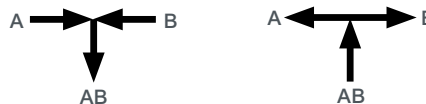
VB-8303 2½"...6" 3-Way Mixing Stem Up Flow is B Port to Common Bottom AB Port VB-8303 2½"...6" 3-Way Diverting Stem Up Flow is Common Bottom AB Port to B Port
