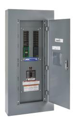
NQ panelboards are primarily used for lighting, plug loads, and power distribution up to 600 Amps. These panelboards NQ panels are designed with 200% rated copper neutrals for non-linear loads. (NQ max volts 240 Vac, max 200kA Short Circuit Current)
