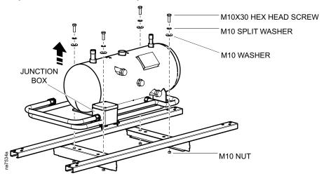
2. Attach the receiver to the mounting bracket from the low temperature accessory kit with hardware from the accessory kit.
