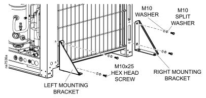
4. Attach the receiver to the mounting brackets and connect the cable conduit.
