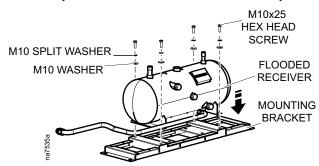
3. Connect the left and right mounting brackets from the accessory kit to the side of the ACCU30X unit.
