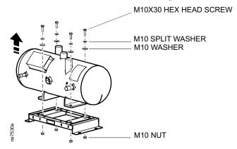
2. Attach the receiver to the mounting bracket from the low temperature accessory kit with hardware from the accessory kit.
