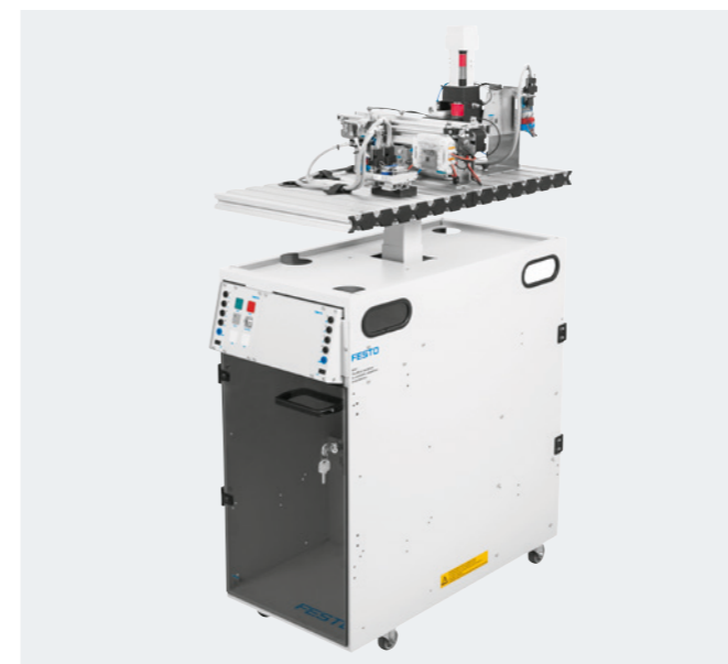
Distributing station with additional equipment
