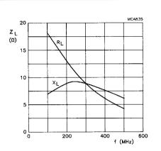
Class-B operation;  $V_{DS} = 28 \text{ V}$ ;  $I_{DQ} = 2 \text{ x } 40 \text{ mA}$ ;  $P_1 = 40 \text{ W}.$
