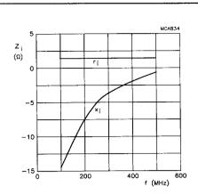
Class-B operation;  $V_{DS} = 28 \text{ V}$ ;  $I_{DQ} = 2 \text{ x } 40 \text{ mA}$ ;  $P_1 = 40 \text{ W}.$
