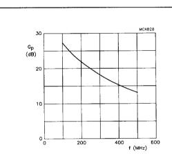
Class-B operation;  $V_{DS} = 28 \text{ V}$ ;  $I_{DQ} = 2 \text{ x } 40 \text{ mA}$ ;  $P_1 = 40 \text{ W}.$
