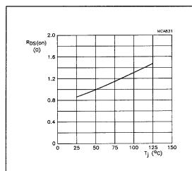
$I_D = 1.2 \text{ A}; V_{GS} = 10 \text{ V}.$
