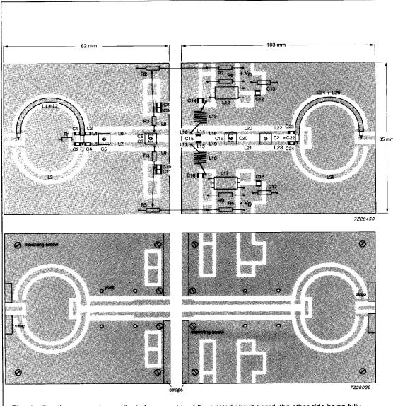
The circuit and components are situated on one side of the printed circuit board, the other side being fully metallized, to serve as a ground plane. Earth connections are made by means of copper straps and hollow rivets for a direct contact between upper and lower sheets.
