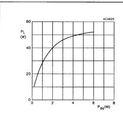
Class-B operation;  $V_{DS} = 28 \text{ V}$ ;  $I_{DQ} = 2 \text{ x 40 mA}$ ;  $Z_L = 4.2 + j6.2 \Omega$  (per section); f = 500 MHz.
