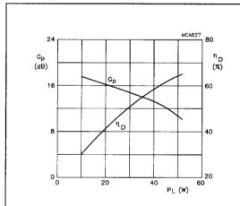
Class-B operation;  $V_{DS} = 28 \text{ V}$ ;  $I_{DQ} = 2 \text{ x } 40 \text{ mA}$ ;  $Z_L = 4.2 + j6.2 \Omega$  (per section); f = 500 MHz.
