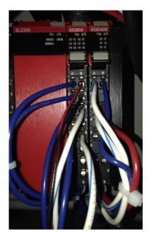
Image of NX CPU, SID800 input, SOH400 output.
