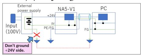
Measure 2 (Isolate the external power supply and NA5-V1)
