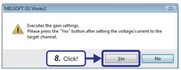
**8.** Apply the gain voltage or current to the terminal of the corresponding channel, and click the [Yes] button.
