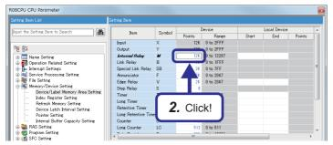
**2.** Click "Points" of "Internal Relay" (M) in the "Device" column to move the cursor.
