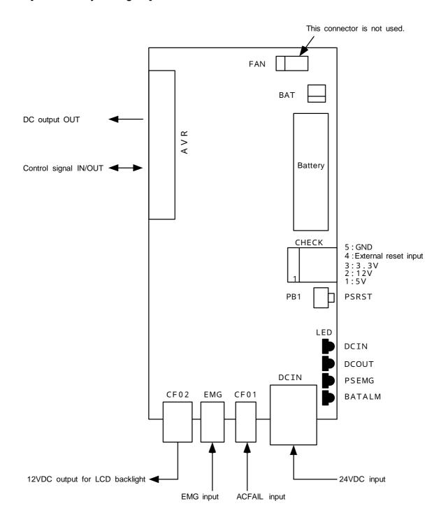
PSRST: System reset (do not press during normal system operation)
