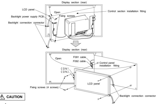
Incorrect connections may damage the devices, so connect the cables to the specified connectors.
