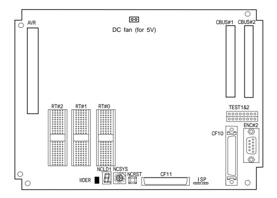
TEST 1 & 2: Test pins for maintenance and service
