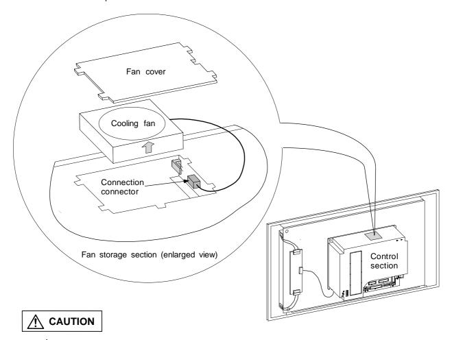
Do not replace the cooling fan while the power is ON.
