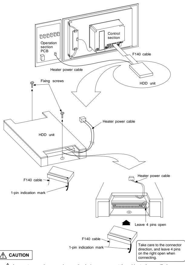
Incorrect connections may damage the devices, so connect the cables to the specified connectors
