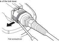
3) The external cable can be removed by pulling the whole plug connector while shifting the coupling of the plug connector to the cable side
