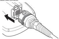
3) After inserting the connector, push the lock lever. The connectors are locked after the lever is pushed into.
