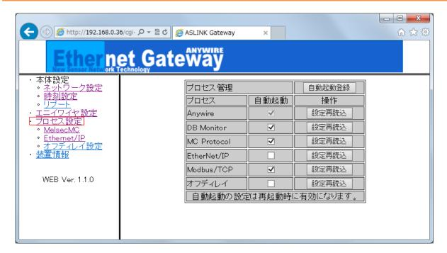
The point number setting for AnyWireASLINK, and SLMP (MC protocol) setting, EtherNet and IP settings can be applied in real time from this screen.
