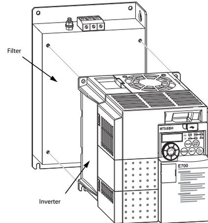
To fix the filter-inverter unit on the cabinet back panel use proper screws (not provided with the filter). For correct filter performance the filter should electrically bond to the cabinet back panel which needs to have proper connection to earth. If needed please remove the paint under the filter footprint.
