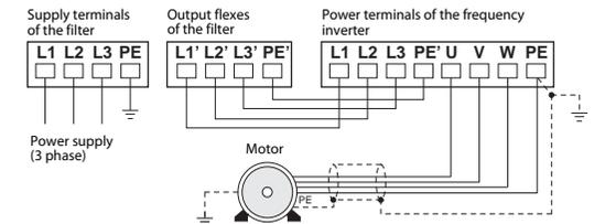
The shielded motor cable must be earthed at both ends in order to reduce radiated noise.
