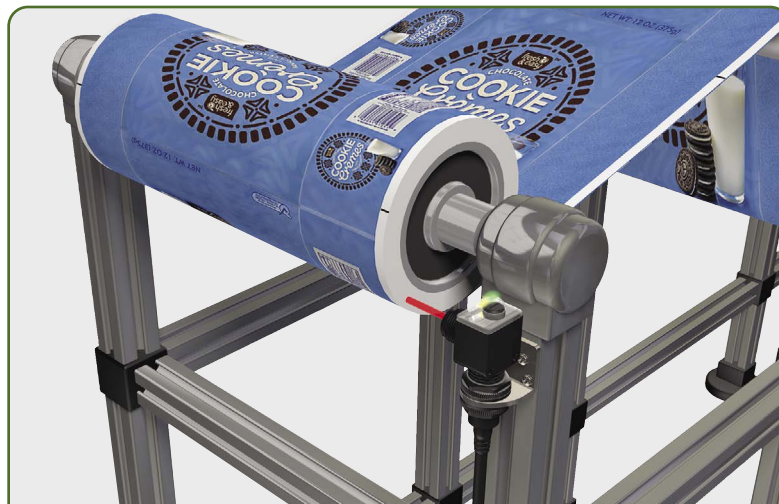
Roll detection - A 42EF RightSight LaserSight monitors a roll of film to indicate low film level.
