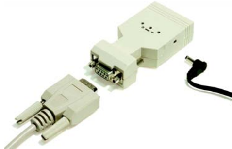
Figure 12 - Connect the PC Receiver Data Port to the Personal Computer
