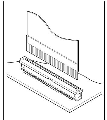
The FAZ connector is SMT type for PC board connector, which is a Zero Insertion Force (ZIF) type for FFC connection with a lead pitch of 1.0 mm.
