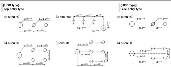
Note: 1. Tolerances are non-cumulative: ± 0.05 mm for all centers. 2. Hole dimensions differ according to the type of PC board and piercing method. The dimensions above should serve as a guideline. Contact JST for details.
