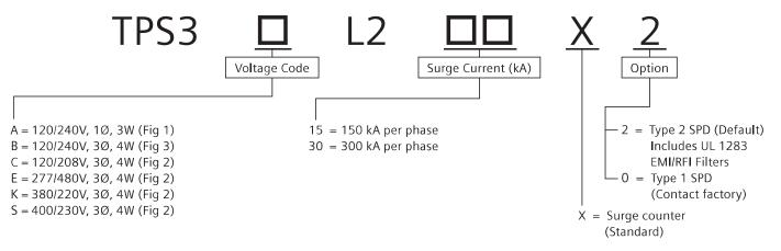
Example: TPS3CL230X2 = 10 Mode Type 2 SPD (Default) for a 208/120V panelboard with a surge current capacity of 300 kA per phase and a surge counter
