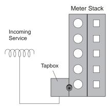
This configuration has no main disconnect and can only be used when there are six or fewer disconnects
