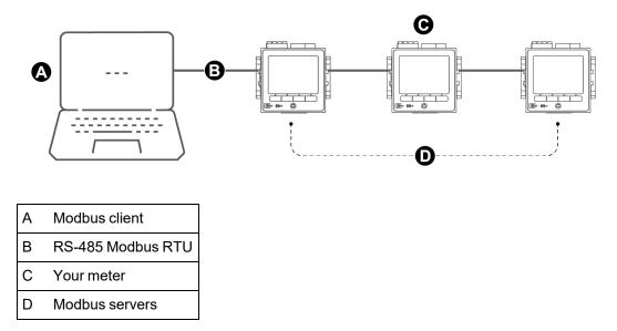
Your meter's serial connection must be wired and configured correctly. The same mode of serial communication must be used for all devices on the network.
