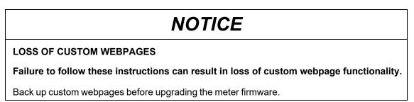
To back up meter webpages, copy the **web** folder to a local folder on the computer using an SFTP client application.
