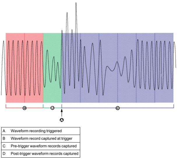
The waveform log set for each triggered recording is equal to the sum of Pre-trigger Records + Post-trigger Records + 1 (where 1 is the actual record when the Waveform Recorder module's Record input was triggered).
