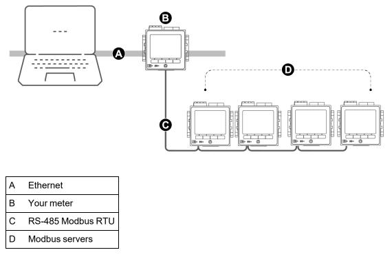
To use the Modbus client-server architecture, add the Modbus server devices using ION Setup.
