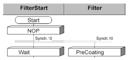
If the synchronization 10 is met by processing the sequence 'FilterStart', it will be attempted to start the sequence filter. If this sequence is busy, in manual mode or the preselection hold is active, the start will be stored and executed later. The processing of the sequence 'FilterStart' is continued.
