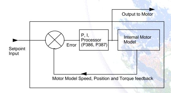
Although there is no position or speed feedback from the motor, the control system is a closed loop system because it compares the internal motor model performance with the desired performance. The system must therefore be carefully set up and stabilised for best performance.
