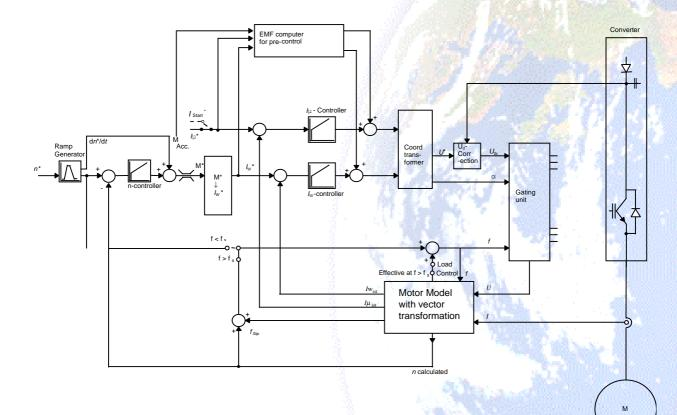
The control system is highly complex, and utilises software and control algorithms developed for other, larger Siemens drives together with an extremely fast floating point calculator.
