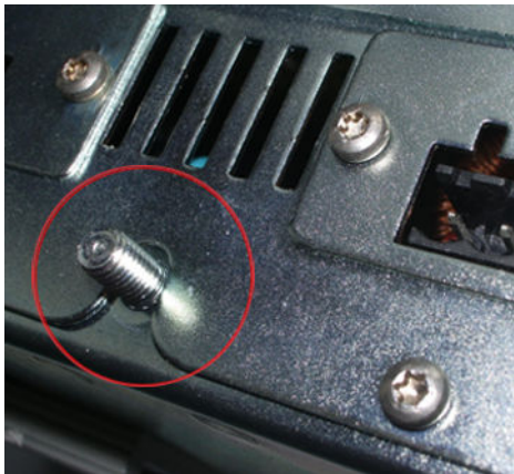
Figure 6-1 Grounding bolts on the bottom of the X-300EEC housing
