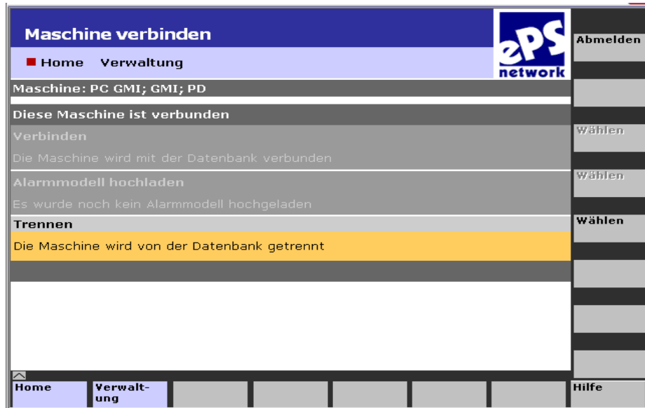
Fig. 7-10: Disconnecting a machine on the HMI
