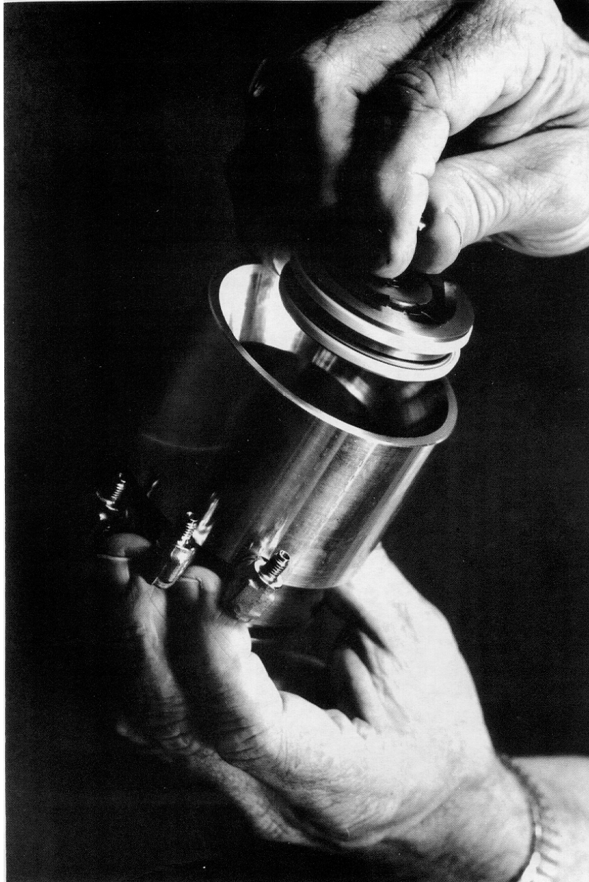
Figure 4-36: Inserting Piston Assembly (15 and 18) into Base (16)
