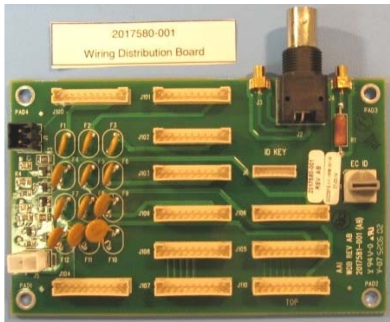
Figure 2-39: Wiring Distribution Board
