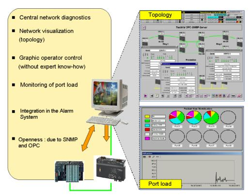
SNMP (Simple Network Management Protocol) is a protocol specially designed to administer TCP/IP networks and has been used for years in the IT world for diagnostics in TCP/IP networks. Switches such as the OSM/ESM also support SNMP. The network components and/or DTEs in Ethernet make their status available with the **SNMP OPC server**.
