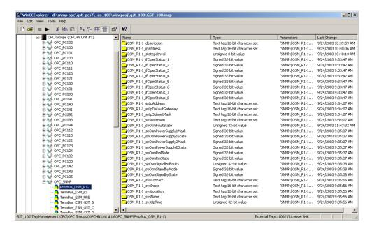
Then adapt the data types of all variables that will be configured later in Alarm Logging (for example ,...\_snOsmFaultState'), where necessary from signed to a signed to allow bit-by-bit evaluation of the alarms in WinCC.
