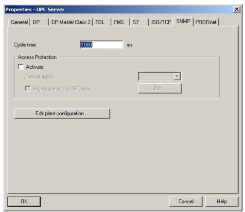
If necessary, the cycle time can be changed in the first box. The cycle time specifies the minimum time in which the variables of the SNMP OPC server can be polled. With the "Access Protection" option, variable access can be controlled (read, write).
