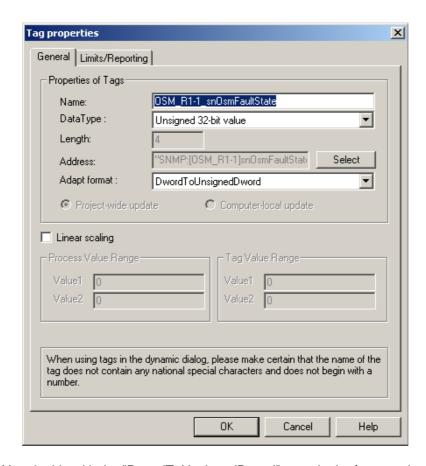
You do this with the "DwordToUnsignedDword" entry in the format adaptation for the example of a 32-bit variable shown above.
