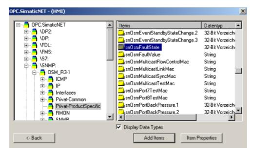
Create a variable in the data manager for each OPC item to be monitored. In the case of the OSM/ESM, the variables "&statepathval()" for connection monitoring and "snOsmFaultState" for fault state monitoring are suitable because error information compression can be used on the device with these variables. In the simplest situation, create a variable in the data manager manually for each OSM/ESM in the network:
