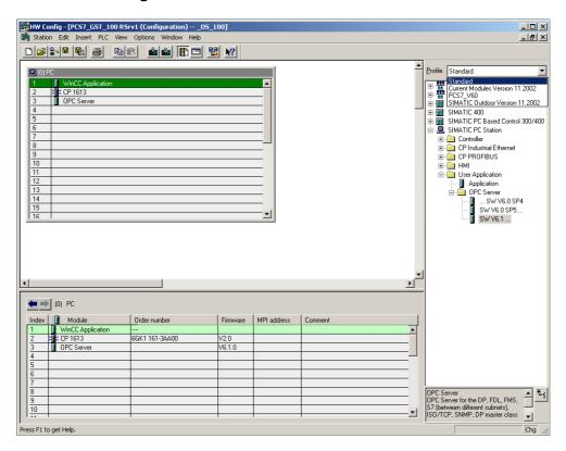
To configure the OPC server, double-click on the "OPC Server" row. The properties dialog of the OPC server opens. Select the "SNMP" tab. The following page is displayed:
