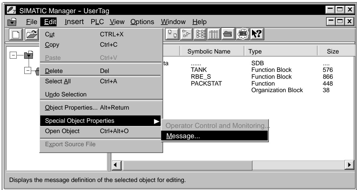
Figure 4-19 Selecting Alarm Messaging
