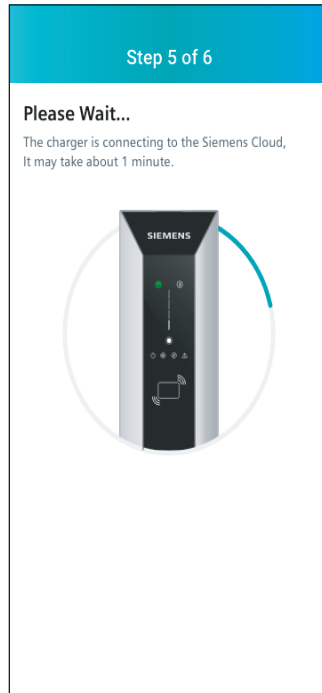
Wait for the charger to connect with the Siemens Cloud. For information about the LED lights during commissioning, see the Wi-Fi LED Light Sequence When Adding a Charger table under section 5.2 above.
