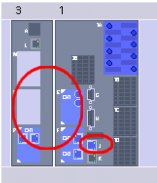
Figure 5-68 Inserting an Ethernet Module
