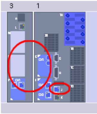
Figure 5-48 Inserting an Ethernet Module
