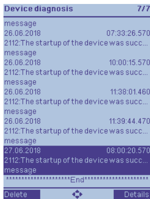
Figure 3-21 Reading the Device-Diagnosis Log on the On-Site Operation Panel of the Device
