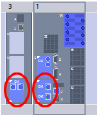
Figure 5-63 Insertion Position for a USART Module
